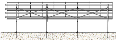
Typical Solar Panel Framing Back View
